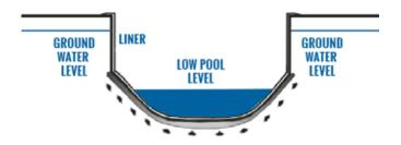
The final area of your pool equipment and plumbing that will require your attention is the Sump Well. It is installed to deal with high water tables or surface drainage which might migrate to the pool area.
